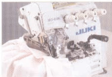
● For gathering MO-6914S-BE6-327/S162 (S162: Swing-type gathering device)
