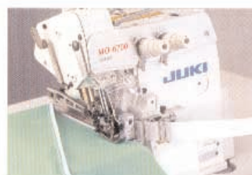
● For rolling-in tape MO-6745S-ED4-360/N077 (N077: Clean finish top and bottom)
